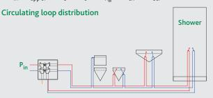
For a detailed calculation of the pressure drops within the loop circuit, please refer to the H. Cross method.
